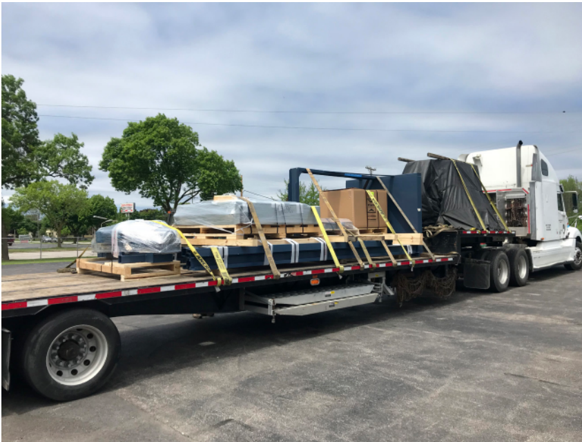
Space is needed to unload, stage, organize, and assemble major VRC components safely.
