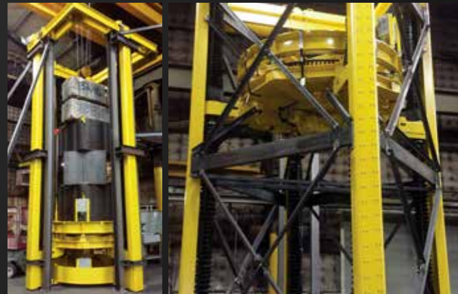
University Research – High-Capacity Lift – Custom 4-Post VRC This precise vertical and circular motion lift is installed in a scientific accelerator facility for nuclear science. 26,000 lbs. lifting capacity; 19' lift travel; 5' per minute travel speed.
