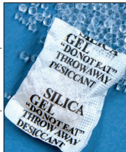
Place Inside Control Enclosure Figure 20-5
