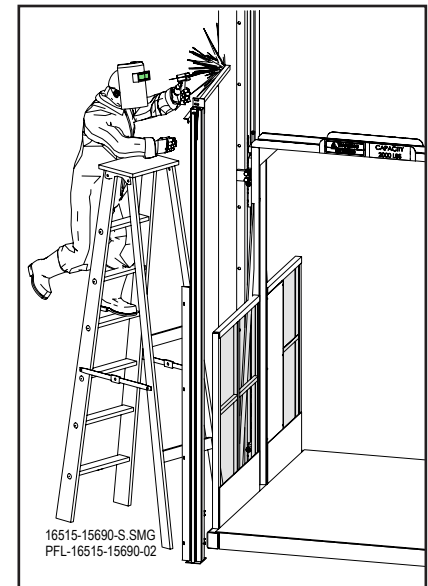
Temporarily Brace Gate Post Figure 21
