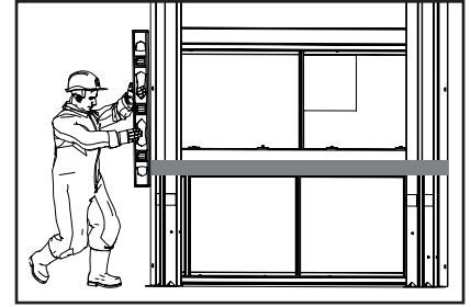
Plumb the Gate Figure 19
