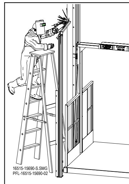
Temporarily Brace Gate Post Figure 28
