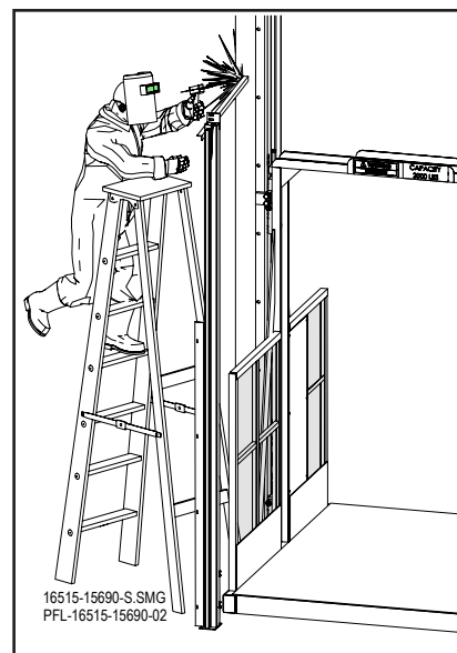
Temporarily Brace Gate Post Figure 24
