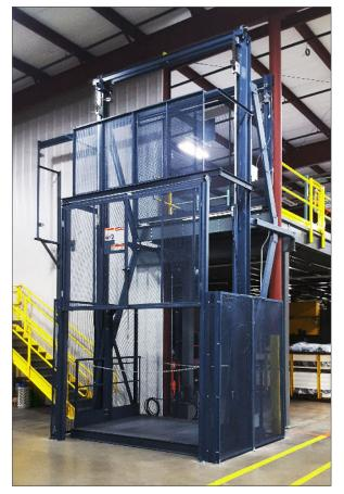
A torsion bar links the cylinders to equalize the load and ensure the carriage remains level.
