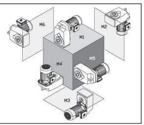
Motor and Gear Reducer Orientations Figure 11-5
