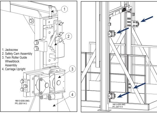
Safety Cam and Twin Roller Guide Location Figure 7-5
