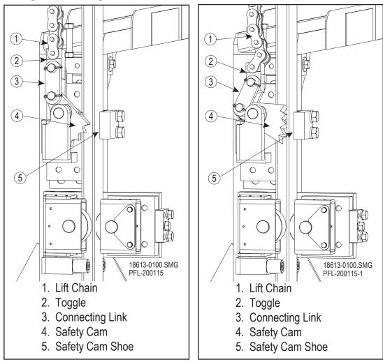
Safety Cam Disengaged Figure 7-7
