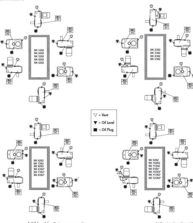
\* Oil level for 3 stage gear units
