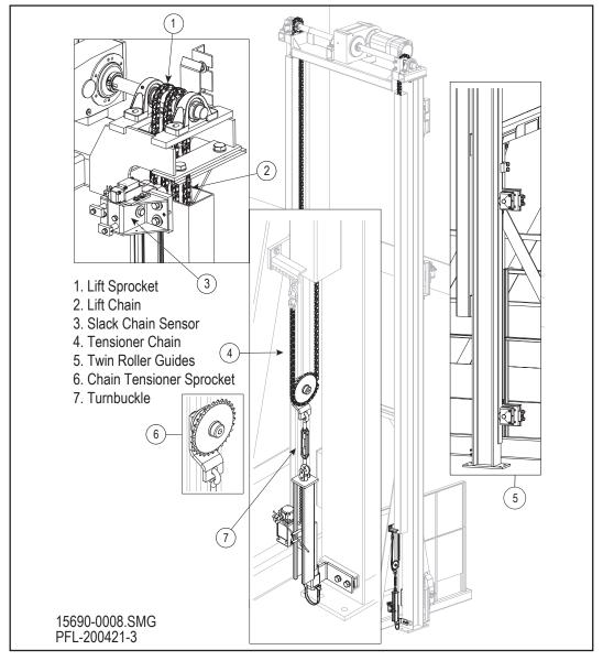
Lift Chain Tensioner and Slack Chain Sensor Figure 9-5
