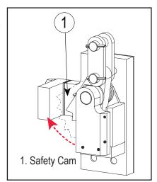
Lubricate and Rotate Safety Cam Figure 18-3
