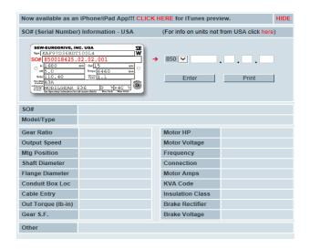
With the SEW Eurodrive SO# (on motor nameplate) the SEW website will indicate the connection diagram number (i.e. connection R72B)
