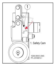
Lubricate and Rotate Safety Cam Figure 18-3
