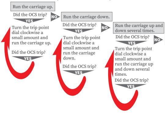
The OCS is properly adjusted.
