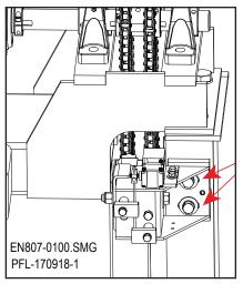
Attach the Slack Chain Sensor Figure 12-45
