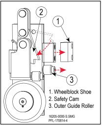
Rotate the Safety Cam Figure 12-13
