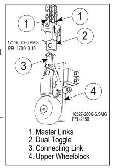
Attach the Upper Wheelblock to the Lift Chains Figure 12-37
