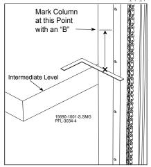
Intermediate Level Limit Switch Position Figure 14-18
