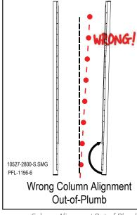
Column Alignment Out-of-Plumb Figure 12-25
