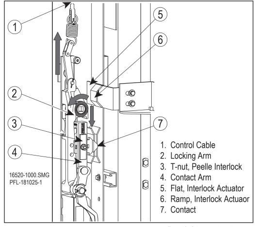
Peelle Interlock Open Position Figure 17-8
