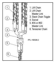
Attach the Tensioner Chain to the Lift Chain Figure 12-35
