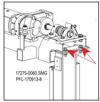
Tighten and Torque Hex Bolts Figure 12-32
