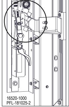
Peelle Interlock Closed Position Figure 17-9
