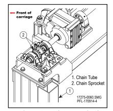
Drop the Tensioner Chain Down the Chain Tube Figure 12-36
