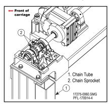
Place a Section Over the Chain Sprocket Figure 12-34
