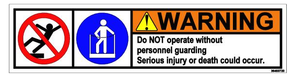
(SIGNAGE LOCATION - Located on all carriage handrails and/or side guards.)
