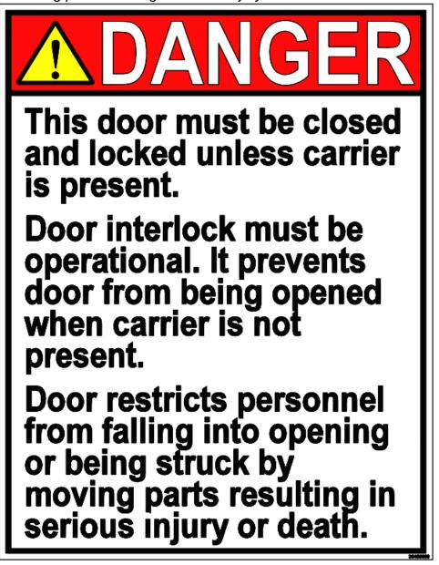
(SIGNAGE LOCATION - Located on or near the gate or door handle or mid-height on vertically sliding doors.)
