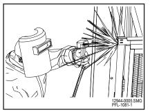
Weld Gate Header to Gate Posts Figure 16-17
