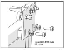
Install Interlock Keeper Assembly Figure 16-28
