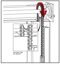
Thread Chain Over the Sprockets Figure 16-53
