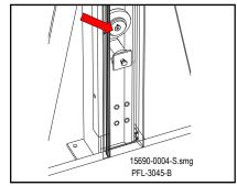
Tighten Mounting Bolt Figure 15-3
