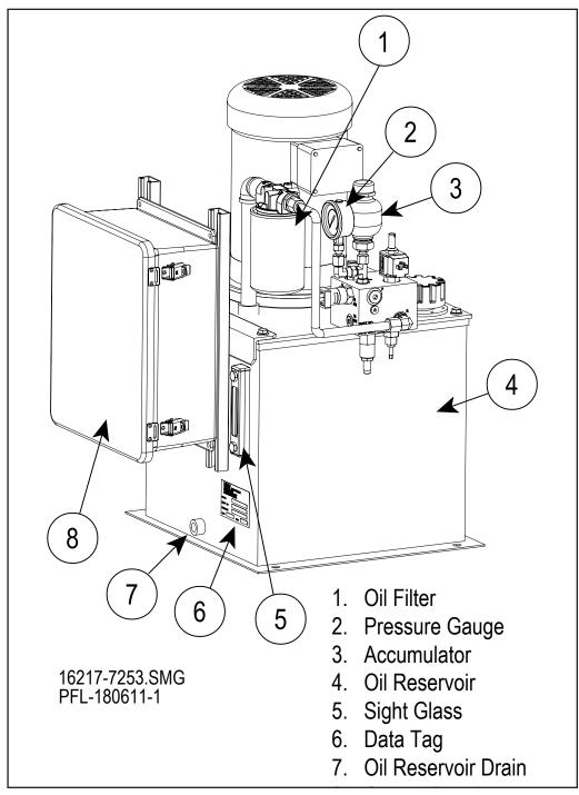
Components of Hydraulic Pump Figure 21-6
