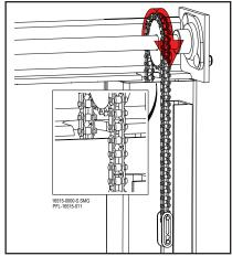
Thread Chain Over the Sprockets Figure 16-85
