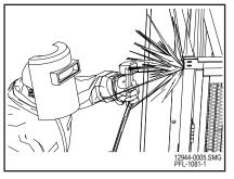
Weld Gate Header to Gate Posts Figure 16-92
