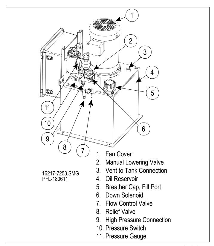
Components of Hydraulic Pump Figure 21-7
