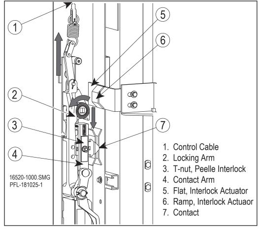
Peelle Interlock Open Position Figure 17-8
