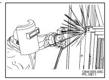
Weld Gate Header to Gate Posts Figure 16-47
