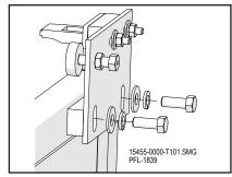
Install Interlock Keeper Assembly Figure 16-9
