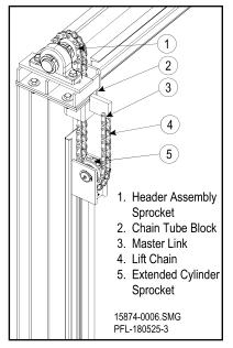
Drop the Lift Chain Down the Chain Tube Block Figure 12-34
