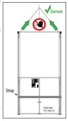
Secure and Lift Gate Assembly Figure 16-74
