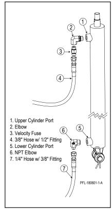
Connect Hydraulic Hose to Cylinder Figure 21-4
