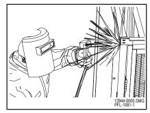
Weld Gate Header to Gate Posts Figure 16-60
