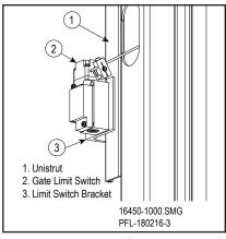
Attach Gate Limit Switch Figure 16-95
