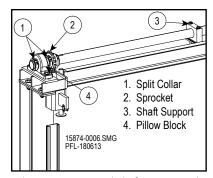
Tighten Setscrews and Shaft Support Bolts Figure 12-36
