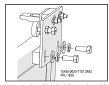
Install Interlock Keeper Assembly Figure 16-18
