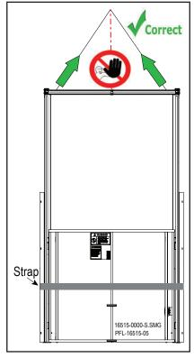
Secure and Lift Gate Assembly Figure 16-44
