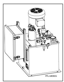
Hydraulic Pump and Motor Location Figure 21-1
