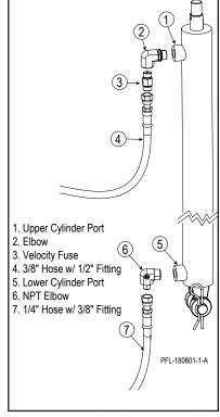
Connect Hydraulic Hose to Cylinder Figure 21-2
