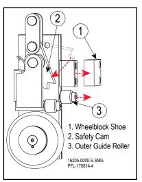
Rotate the Safety Cam Figure 12-12
