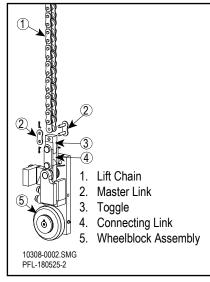
Attach the Lift Chain to the Wheelblock Figure 12-35
