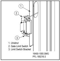
Attach Gate Limit Switch Figure 16-80
