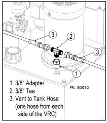
Connect Vent to Tank Hydraulic Hoses Figure 21-9
