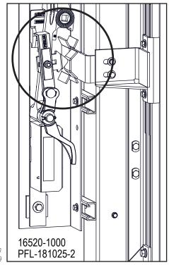
Peelle Interlock Closed Position Figure 17-9
