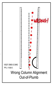
Column Alignment Out-of-Plumb Figure 12-26
