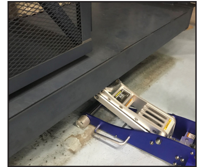
Floor Jack Placement Figure 3
