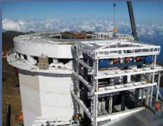
Telescope Lift – Custom Designed 4-Post VRC 19' x 19' lift carriage and dual motor drive transport the telescope's delicate mirror. 54,000 lbs. lifting capacity (44,000 lb. mirror/10,000 lb. carriage); 76' lift travel; 5' per minute travel speed.
