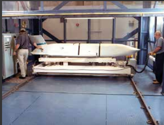
Missile Work Platform – Custom Screw Lift Vertical travel is controlled via screw lifts. Travels laterally on 18" wheels. 6,500 lbs. lifting capacity.
