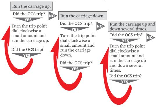
The OCS is properly adjusted.
