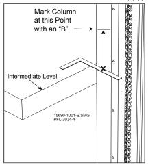
Intermediate Level Limit Switch Position Figure 14-18
