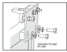
Install Interlock Keeper Assembly Figure 16-18
