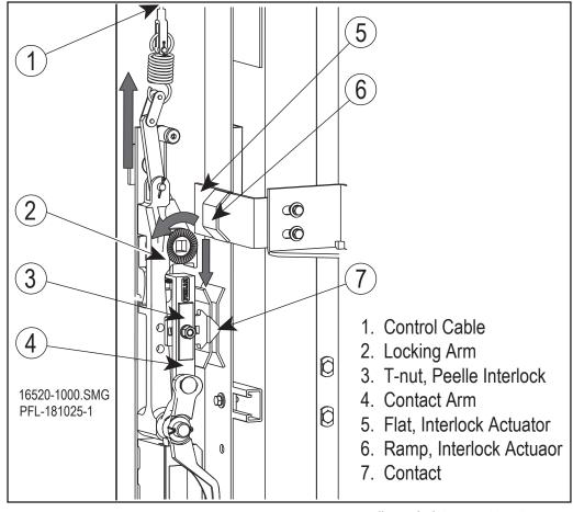
Peelle Interlock Open Position Figure 17-8
