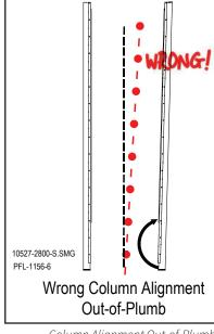
Column Alignment Out-of-Plumb Figure 12-17
