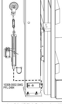
Install the Lift Chain Tensioner Assembly Figure 12-46
