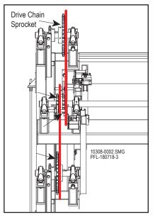
Verify Sprocket Alignment Figure 12-37
