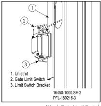
Attach Gate Limit Switch Figure 16-95
