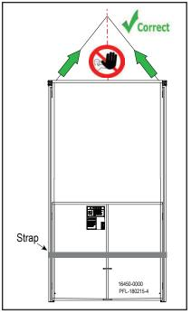
Secure and Lift Gate Assembly Figure 16-74
