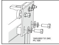
Install Interlock Keeper Assembly Figure 16-9
