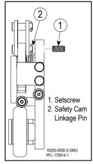
Insert Setscrew Figure 12-12 Insert Setscrew Figure 12-13
