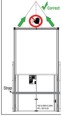
Secure and Lift Gate Assembly Figure 16-44
