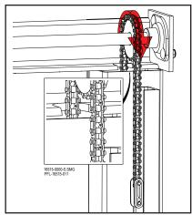
Thread Chain Over the Sprockets Figure 16-85
