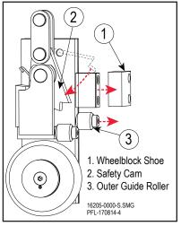
Rotate the Safety Cam Figure 12-11
