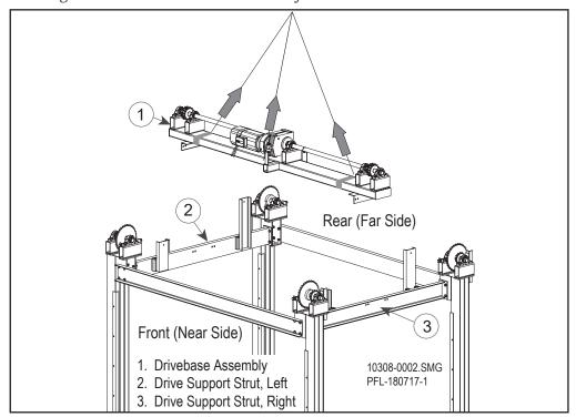
Drivebase Assembly Placement Figure 12-33
