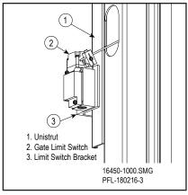
Attach Gate Limit Switch Figure 16-80
