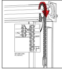
Thread Chain Over the Sprockets Figure 16-53
