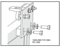
Install Interlock Keeper Assembly Figure 16-28
