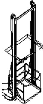
**4.1.1** This design type, as illustrated above, places the carriage between the guide beams and applies the load forces in the vertical direction along the length of the guide beams.
